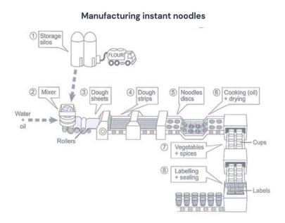
The diagram illustrates the process by which instant noodles are produced.
